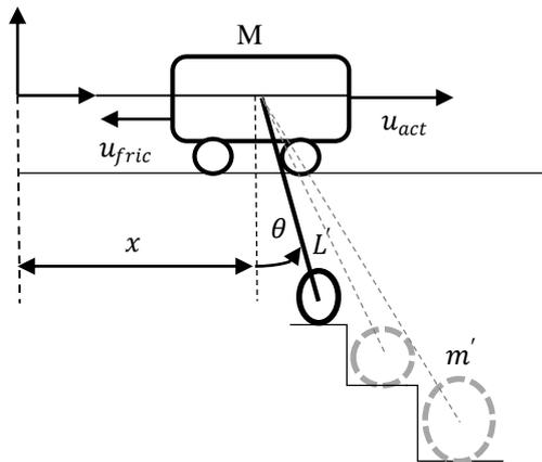
Fig. 2. The model of crane system.
