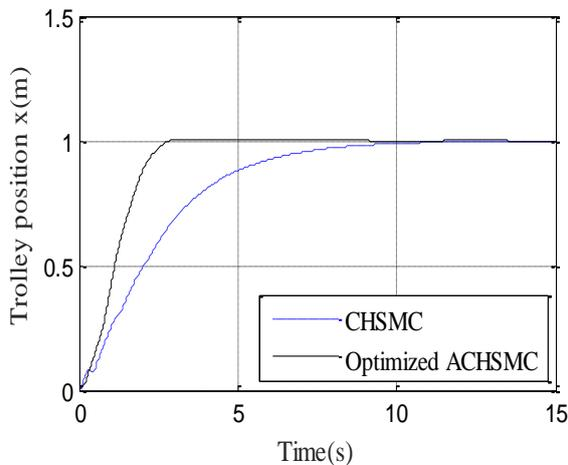
**Fig. 4.** Crane trolley position.
