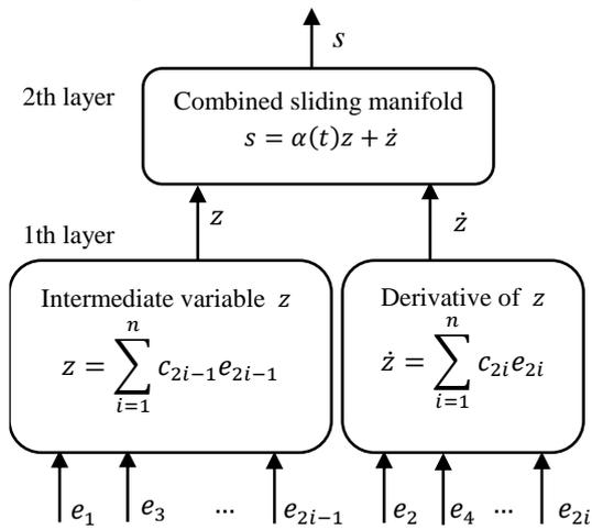
Fig. 1. Combined hierarchical sliding manifold.
