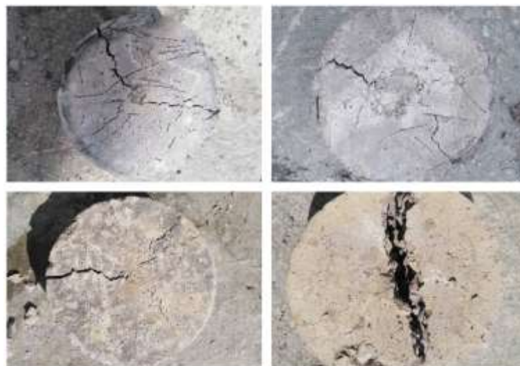
Fig. 2. Images of concrete specimens after hammer impact test
