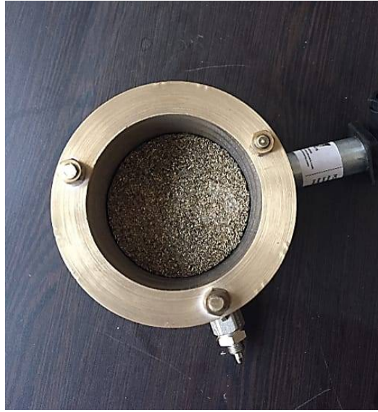
FIGURE 3. Positioning porous rock on top of the sample.
