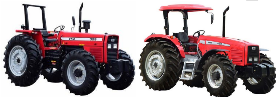
Fig.1. ITM399 without turbo charger (Left) and ITM 4120 with turbo charger (Right) tractors
