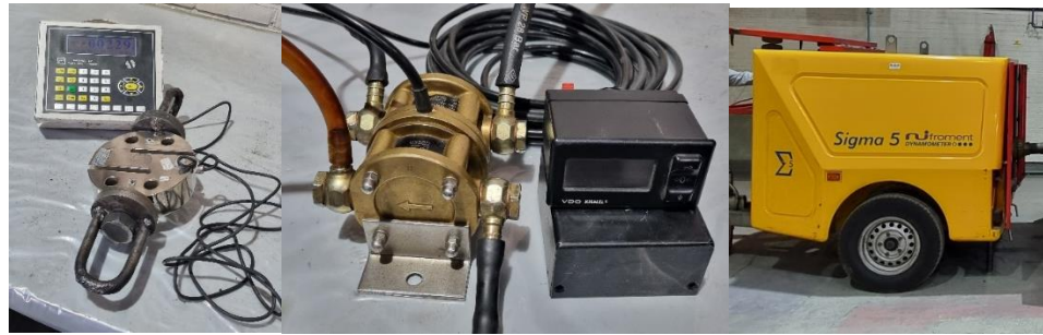
Fig. 2. Load cell, fuel gauge and dynamometer used in the traction test and fuel consumption of tractors
