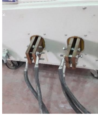
Fig. 11. Output terminals of single-phase transformer used for current injection test.
