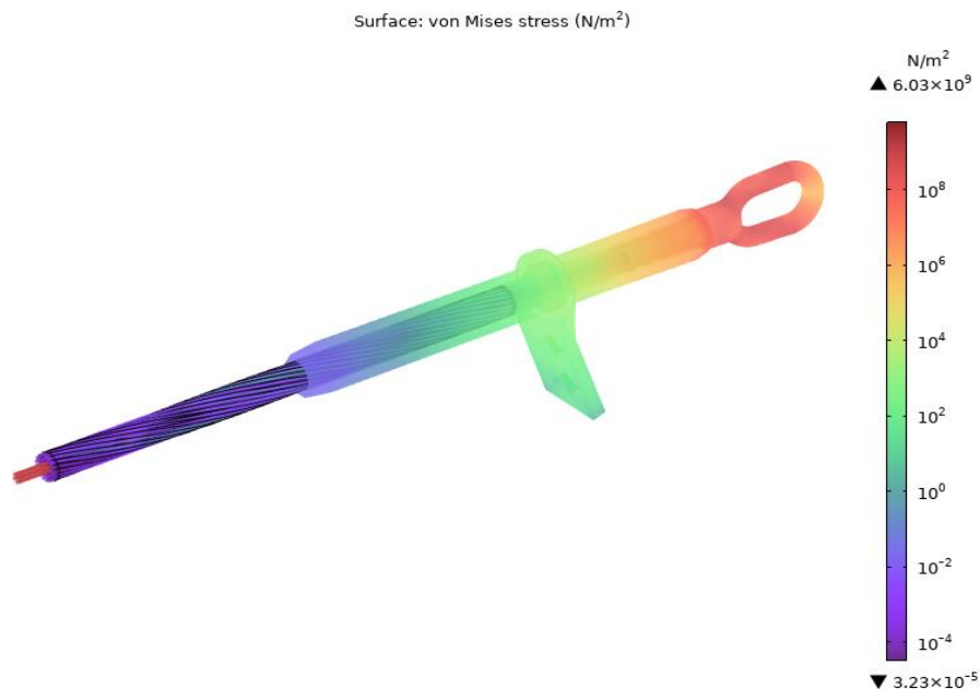
Fig. 7. Von Mises stress distribution under 77.3 kN .
