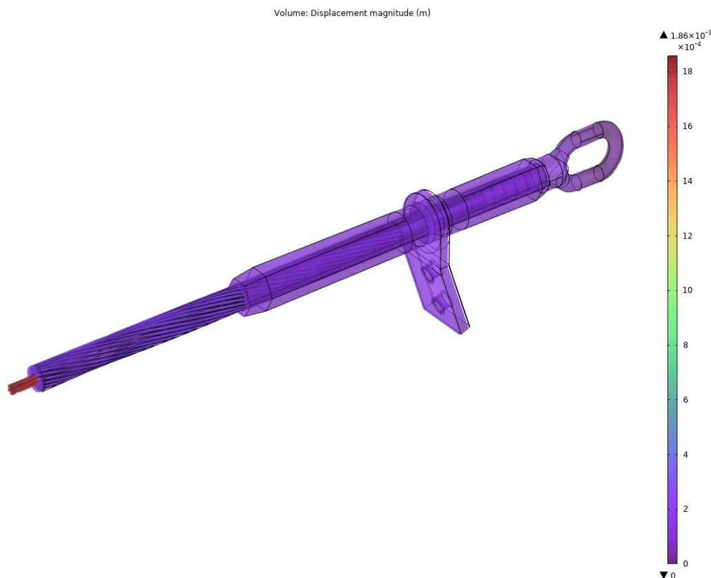
Fig. 8. The displacement of the clamp-conductor system under the 77.3 kN .
