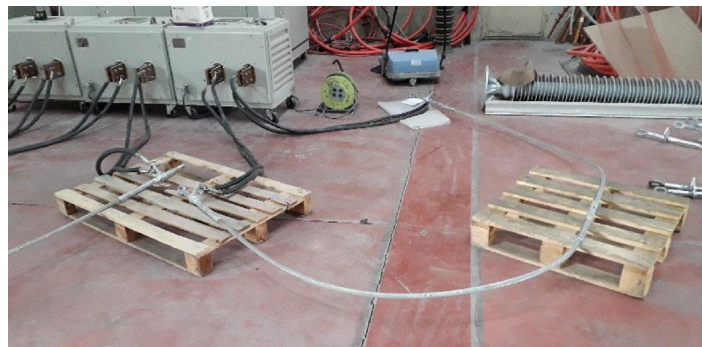
Fig. 13. A view of studied sample ready for current injection test.
