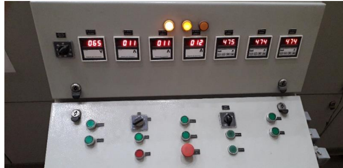
Fig. 12. Voltage regulator control panel used for current injection test.
