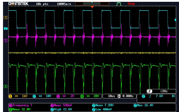
Fig. 12. Experimental waveforms; Ch.1 is the output voltage, Ch.2 is push-pull gate voltage, Ch.3 is voltage of compensator, V_{comp} , and Ch.4 is voltage of linear regulator, Q_1 .
